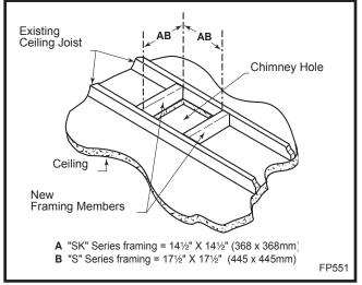
Fig. 12 Typical frame for ceiling chimney hole.
